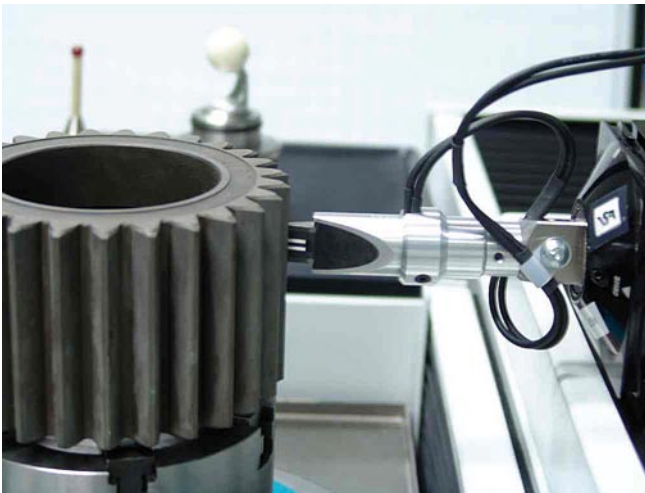
Gear sensor measuring Barkhausen Noise in a gear.
