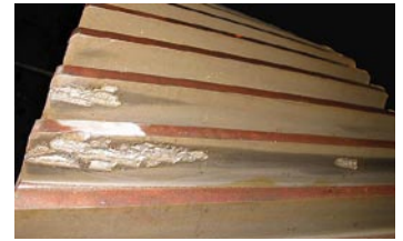
Gear failure caused by grinding burn.
