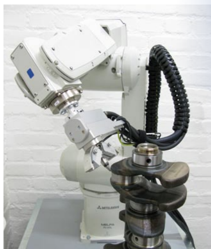
Xstress Robot taking the role of a goniometer.
