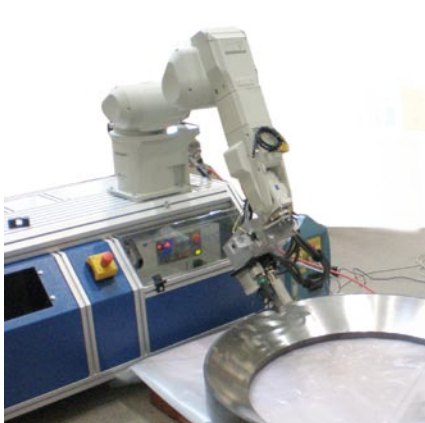
A bearing being measured with Xstress Robot with G2.
