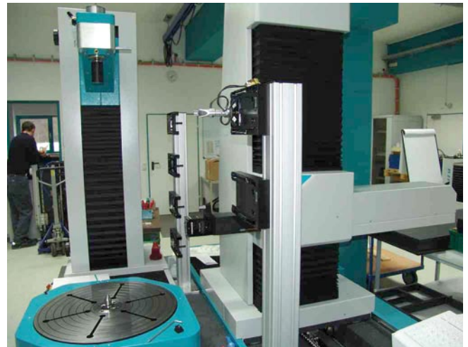
Gear Measuring Machine (GMM) by Wenzel with a gear sensor.
