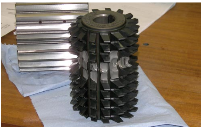
Hob after fatigue crack due to grinding damage.
