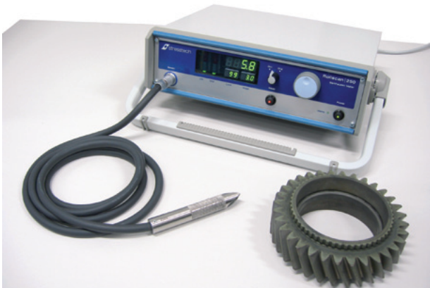
Manual Barkhausen Noise measuring with Rollscan 250
