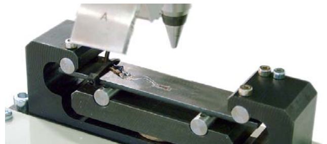
Measuring elasticity constant using strain gages.
