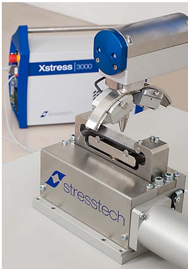
Elasticity constant device (four-point bending device).
