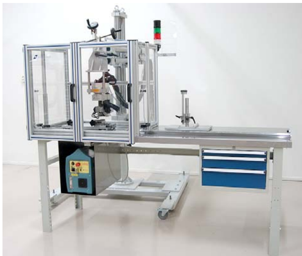
Safety enclosure protecting measurement area on the table for electropolishing.
