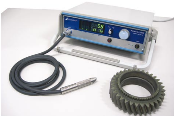
Manual Barkhausen Noise measuring with Rollscan 250
